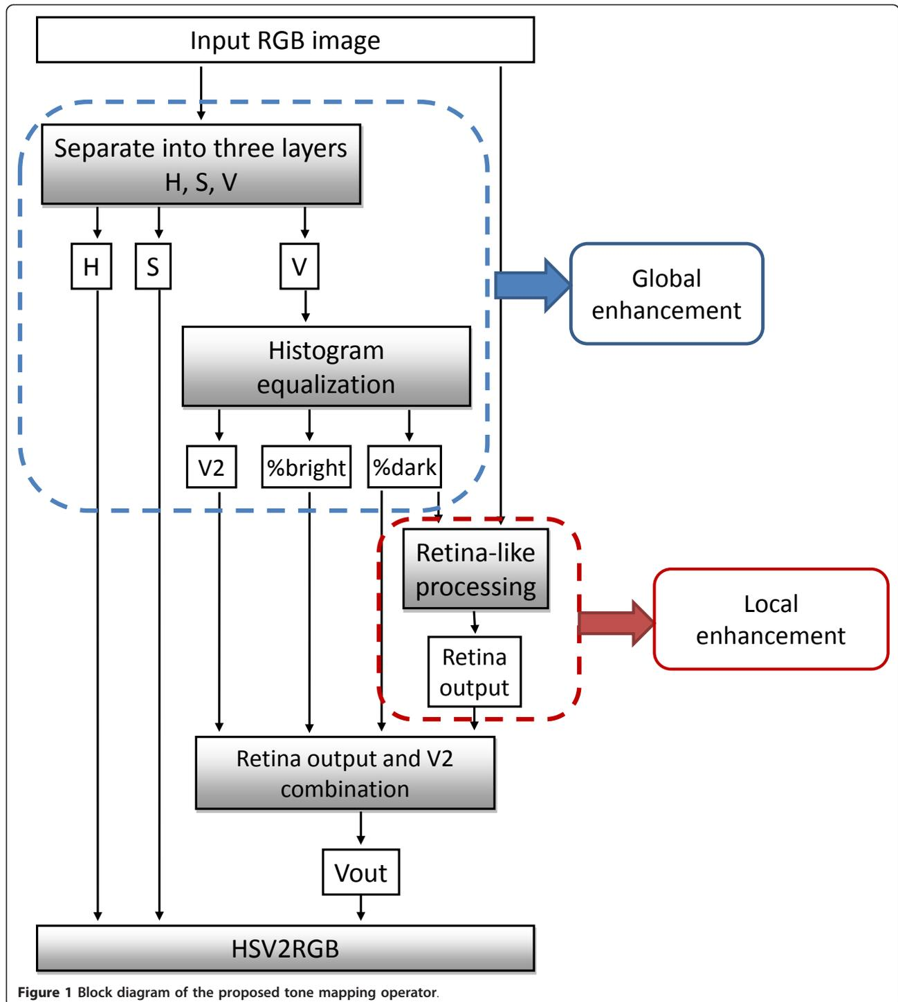
Figure 1 Block diagram of the proposed tone mapping operator.
