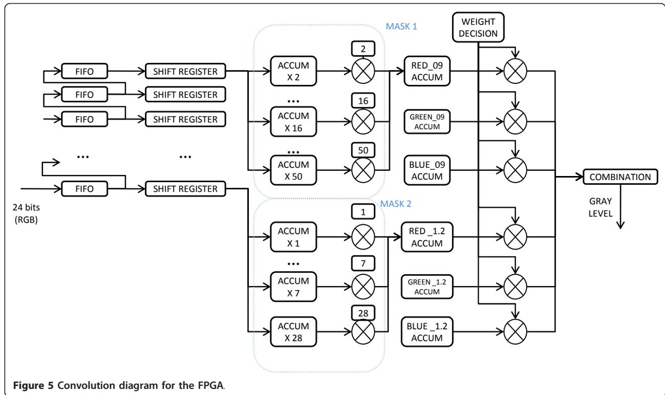
Figure 5 Convolution diagram for the FPGA.
