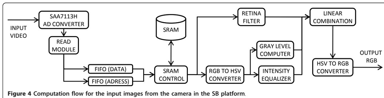
Figure 4 Computation flow for the input images from the camera in the SB platform.
