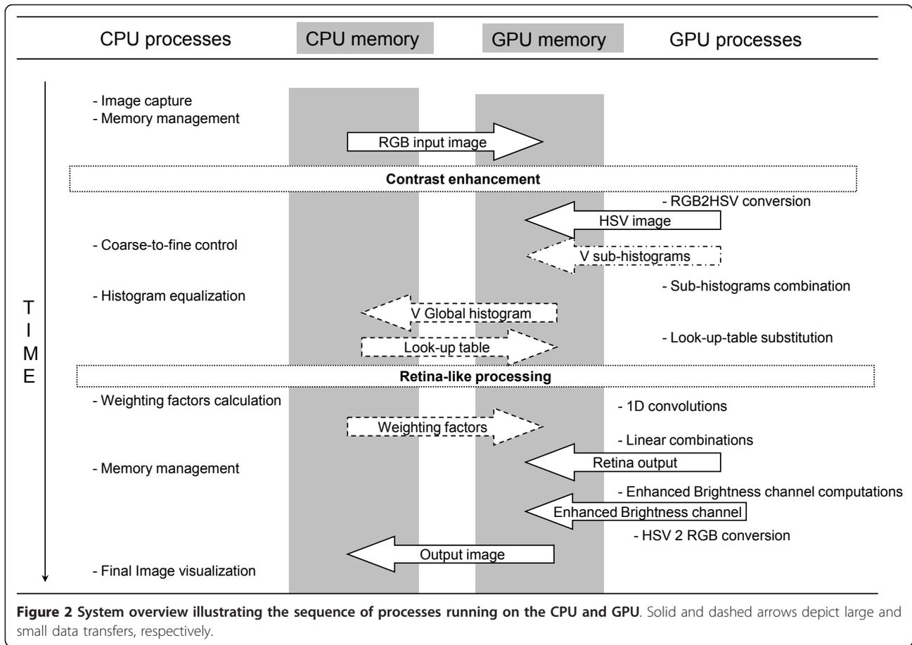
**Figure 2** System overview illustrating the sequence of processes running on the CPU and GPU. Solid and dashed arrows depict large and small data transfers, respectively.
