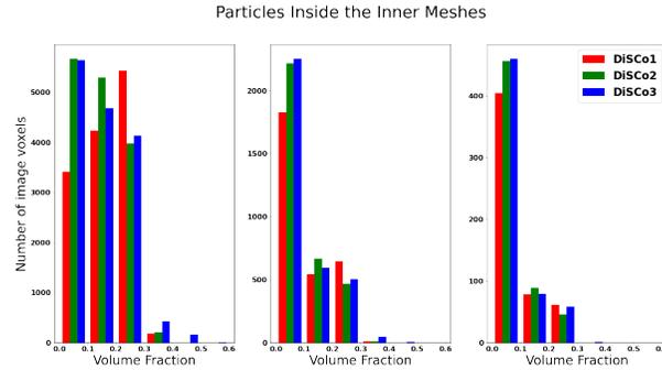
**Fig. 3.** Histograms of the fraction of inner strand fraction for the phantoms DiSCo1 (red), DiSCo2 (green) and DiSCo3 (blue). The voxel size of the image voxel size was set to 25  $\mu\text{m}$  (left), 50  $\mu\text{m}$  (center) and 100  $\mu\text{m}$  (right) isotropic.
