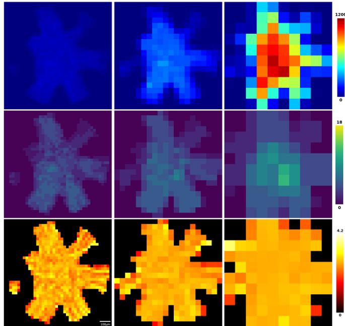
**Fig. 5.** Ground truth strand count map (top), bundle count map (middle) and average strand diameter map in  $\mu m$  (bottom). The voxel size of the image voxel size was set to  $25 \mu m$  (left),  $50 \mu m$  (center) and  $100 \mu m$  (right) isotropic.
