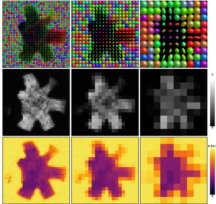
**Fig. 6.** Diffusion tensor estimated from the noiseless DW-MRI signal (top), fractional anisotropy map (middle) and mean diffusivity map (bottom). The mean diffusivity map is reported in  $mm^2s^{-1}unit$ . The voxel size of the image voxel size was set to 25  $\mu\text{m}$  (left), 50  $\mu\text{m}$  (center) and 100  $\mu\text{m}$  (right) isotropic.
