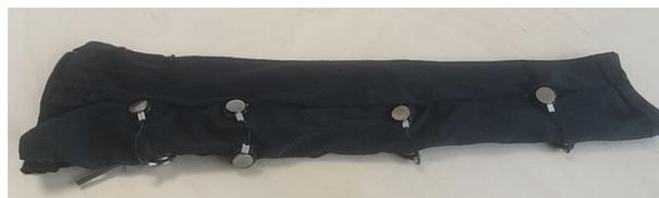
FIGURE 3. Physical prototype of the lymphometer.
