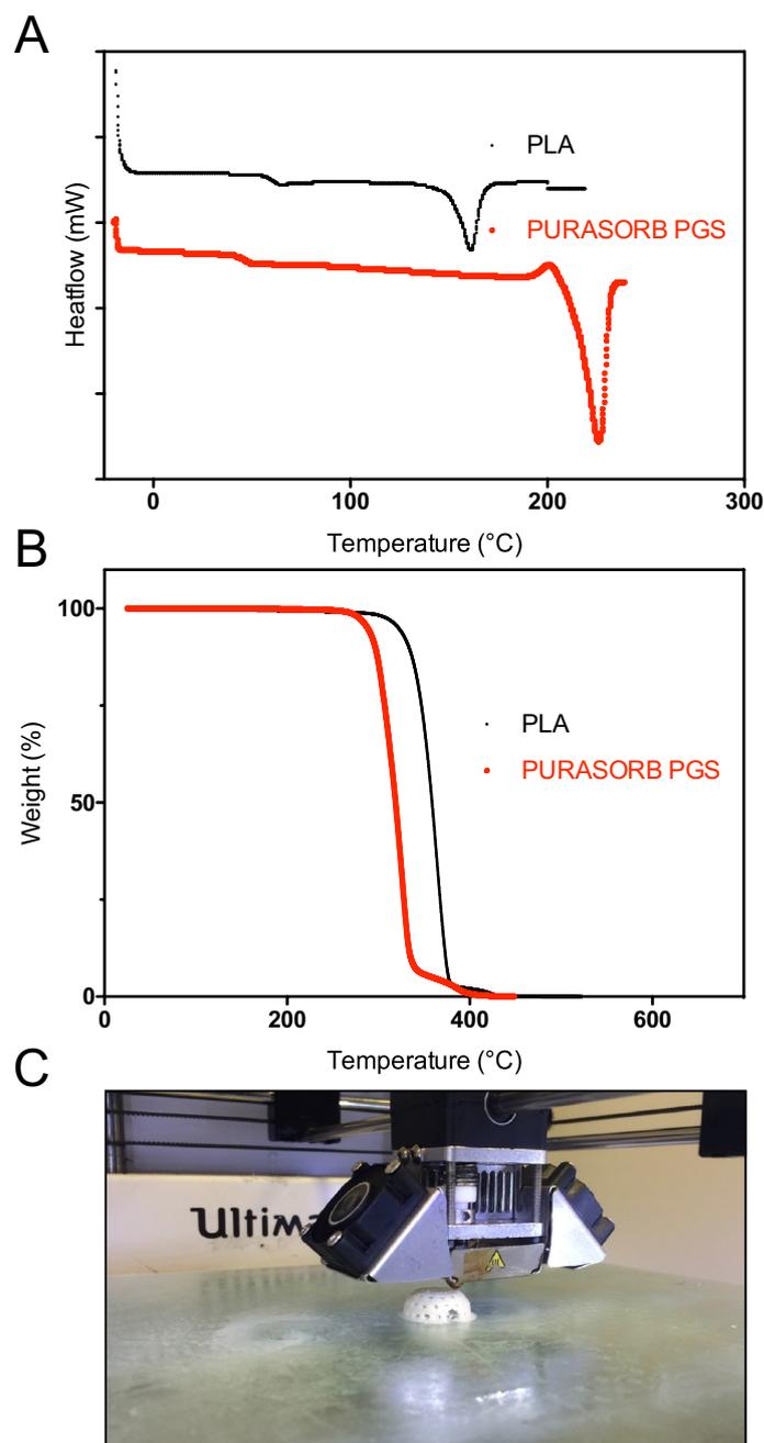
**Figure 1.** Material characterization and construction of TEC model (a) DSC curves of non-printed monofilaments of PLA (black) and PURASORB PGS (red) at a heating rate of 10 °C/min; (b) TGA curves of PLA (black) and PURASORB PGS (red); (c) Representative photomicrograph of TEC sample 3D-printed with PLA material for in vivo experiments.
