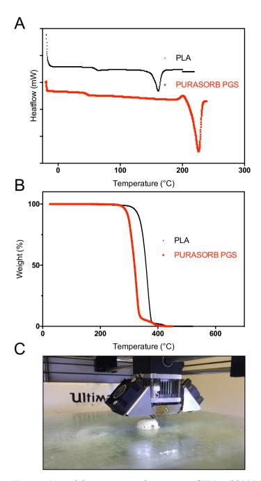
**Figure 1.** Material characterization and construction of TEC model (a) DSC curves of non-printed monofilaments of PLA (black) and PURASORB PGS (red) at a heating rate of 10 °C/min; (b) TGA curves of PLA (black) and PURASORB PGS (red); (c) Representative photomicrograph of TEC sample 3D-printed with PLA material for in vivo experiments.
