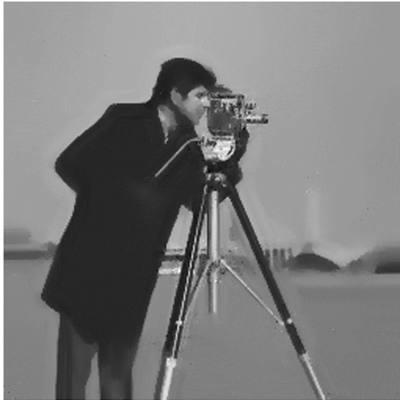
Fig 3. 256×256 denoised Cameraman image under 30db noise. The patch size is 20, K is 9 and \lambda is 0.05. Although the noise is removed, some image details are also eliminated such as building outline and grass on the ground. Besides, the image is blurred. A virtual outline appears around the image edges.
