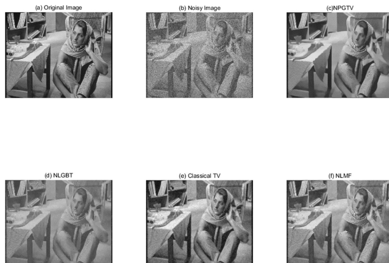
Fig 6. Results of different denoising methods on 576 \times 720 Barbara image. The image is corrupted by the noise at \sigma = 30\text{ dB} . (a): Original image. (b): Noisy image. (c): NPGTV with k = 5 , \lambda = 0.05 , patch size 9 \times 9 . (d): NLGBT algorithm. (e): Classical TV. (f) NLMF with search window size 3 \times 3 , similar widow size 5 \times 5 and the standard deviation is set to 0.1. (The original Barbara image in our paper is taken from Fig 1 in [19] published by the journal PLOS one, which is licensed under the Creative Commons Attribution International License (CC BY 4.0)).
