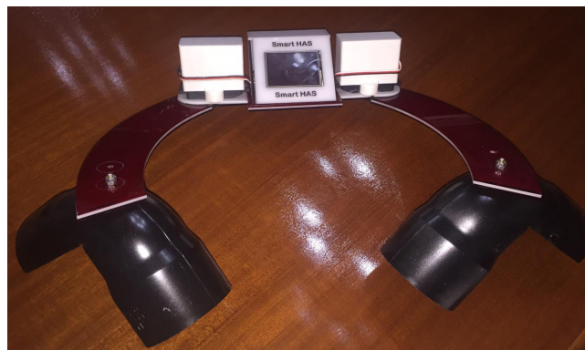
Fig. 3: Smart Hip Abduction Splint (HAS) for Developmental Dysplasia.
