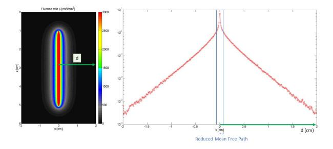
Figure 3. A 2D cross section map (on the left) and 1D line scan plot (on the right) of fluence rate values for a 40 mm length diffuser computed with Monte-Carlo method. At distances below this MFP', the analytical light propagation models become inaccurate.
