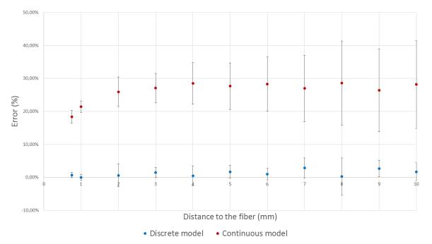
Figure 4. Data points are the mean relative deviations of fluence rate values computed by discrete and continuous methods, calculated for each distance d (0.75 mm to 10 mm) over all six different source lengths. Error bars are standard deviations.
