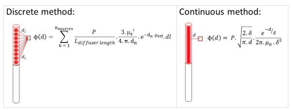
Figure 2: Illustration of the two analytical equations. The discrete method discretizes the diffusing part of the optical fiber as a sum of several light point sources. The continuous method considers the light source as a finite line and computes the fluence rate values using the minimal distance d from the fiber.
