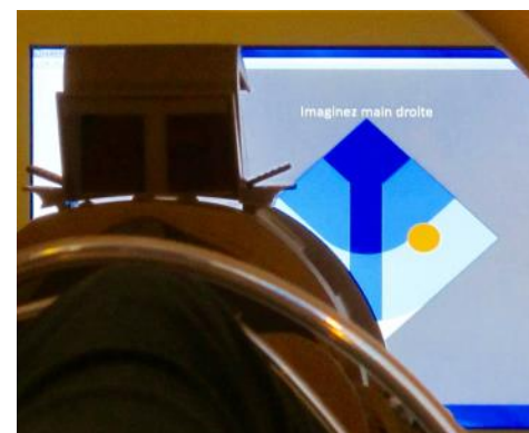
Figure 5. Snapshot of a subject during an experiment. The subject is trying to move the orange disk toward the darkest blue colored area using its brain activity generated by performing motor imagery tasks and measured in real time using EEG and fMRI.
