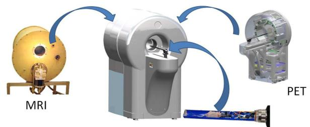
Figure 1: The design of the in-line prototype.
