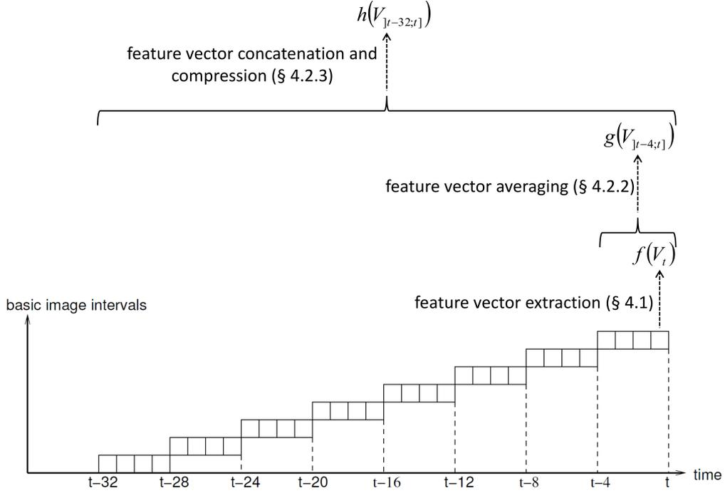
Figure 3: Extracting subsequence feature vectors
