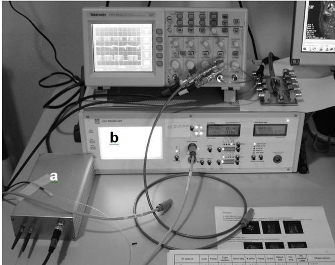
Fig. 1. Optical module (a) connected to a commercial trigger unit (b). The transmitter and receiver fibres and the electrical output coaxial cable are seen in front of the optical module.
