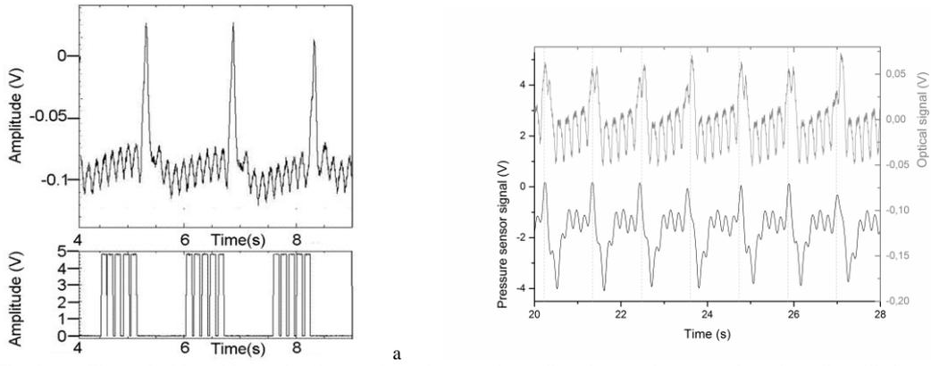
Fig. 4. (a) The optical-based input signal (top) shows large peaks attributed to respiratory cycle and small oscillations to heart motion. The derived gating signal (bottom) from trigger unit outputs is used to synchronize MRI acquisitions. (b) Simultaneous acquisition of optical-based signal (top) and pressure sensor signal (bottom) to monitor respiration and heart motions.
