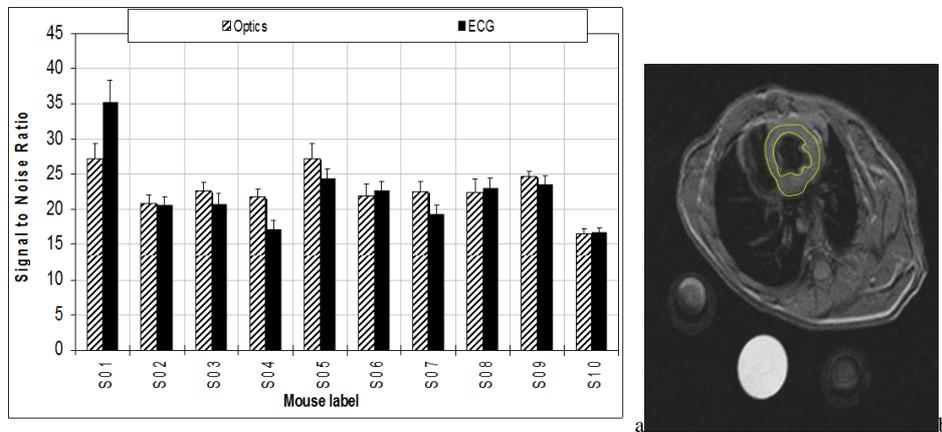
Fig. 8. Black Blood CINE FLASH Sequence. (a) Mean SNR-values measured on myocardium wall with two different methods and for each mouse. Mean SNR-values were  $22.8 \pm 3.1$  and  $22.4 \pm 5.2$  for optics and ECG respectively. (b) Example of MR image acquired with ECG sensor. The ROI matching to the myocardium wall is overlaid on the images.
