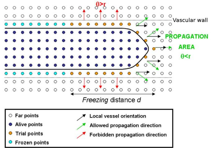
Fig. 2. The restricted and oriented front propagation and its combination with the *Freezing* procedure in 2D space. The front is only allowed to propagate into a restricted area defined by the angular value  $r$ .  $\theta$  is the angle between the direction of the normal to the front  $\vec{n}$  at position  $(x, y, z)$  (red or green arrow) and the local orientation  $\vec{\Gamma}$  (black arrow).
