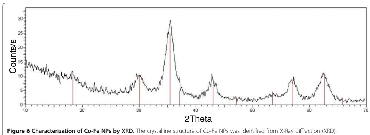
**Figure 6** Characterization of Co-Fe NPs by XRD. The crystalline structure of Co-Fe NPs was identified from X-Ray diffraction (XRD).
