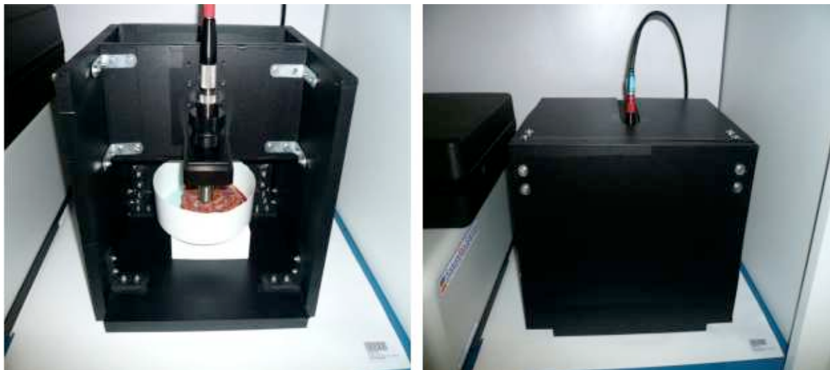
Figure 1: Optical Spectroscopy acquisition device: tumoral kidney is placed under the light source and the spectra are acquired with the black box completely sealed to avoid signal contamination by ambient light.
