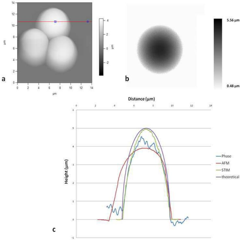
Figure 3: Comparison between different imaging techniques of the  $5\ \mu\text{m}$  spheres. a. the AFM image of the  $5\ \mu\text{m}$  spheres, b. STIM image of the  $5\ \mu\text{m}$  sphere, c. comparison between the experimental profiles (phase, AFM and STIM) and the theoretical prediction.
