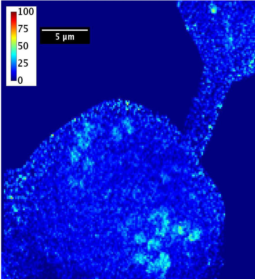
Figure 5: Fully quantitative map showing the projected concentration of Zn in the cell B. The calibration bar is in *ppm*. The map was created by combining the X-ray fluorescence map of Zn and the phase map of the cell B by dividing both images pixel by pixel.
