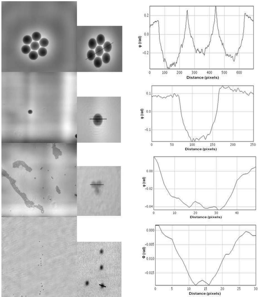
Figure 2: Relative phase maps generated after applying phase retrieval procedure to the certified polystyrene spheres of following diameters:  $10.03 \pm 0.05 \mu\text{m}$ ,  $4.987 \pm 0.040 \mu\text{m}$ ,  $0.994 \pm 0.021 \mu\text{m}$ ,  $400 \pm 4 \text{ nm}$ , together with selected profiles.
