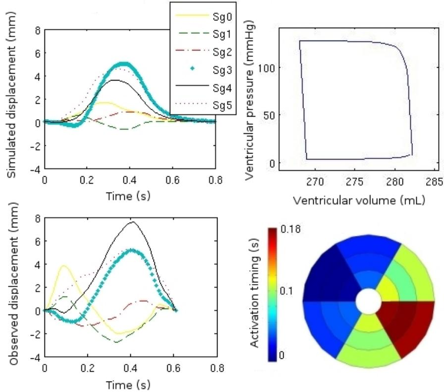
**Fig. 5.** On the left, radial displacement signals of upper segments of the ventricle simulated by the identified model (top) and measured in echography (bottom). On the right, Pressure/Volume cycle simulated by the identified model (top) and bull’s eye diagram of the simulated electrical activation timing for each of the 18 segments (bottom).
