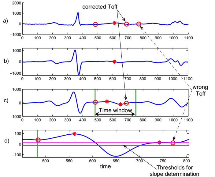
Fig. 4. T wave detection on a sinus beat from the QT database. The upper panel a) presents the original beat ( $W^{2^0}$ ), the second panel b) is the decomposition at level 3 ( $W^{2^3}$ ), and the two last plots, c) and d) are the decompositions at level four ( $W^{2^4}$ ), with different temporal supports.
