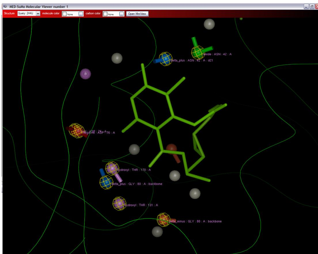
**Figure 8:** A close view around the radical ligand. The eight labelled SCFs (circled in yellow) are shared by all superimposed structures in figure 7. They are located all around the ligand meaning that the similarities concern the whole binding site.
