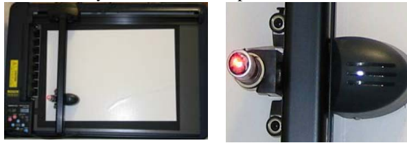
Fig. 2. (a) Pen plotter hung on the wall in front of the MRI scanner (3 meters). (b) Enlargement of the red laser pointer which substituted the colour pen.
