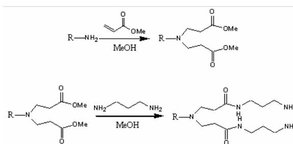
Fig. 1: Successive steps conducted for the dendron synthesis
