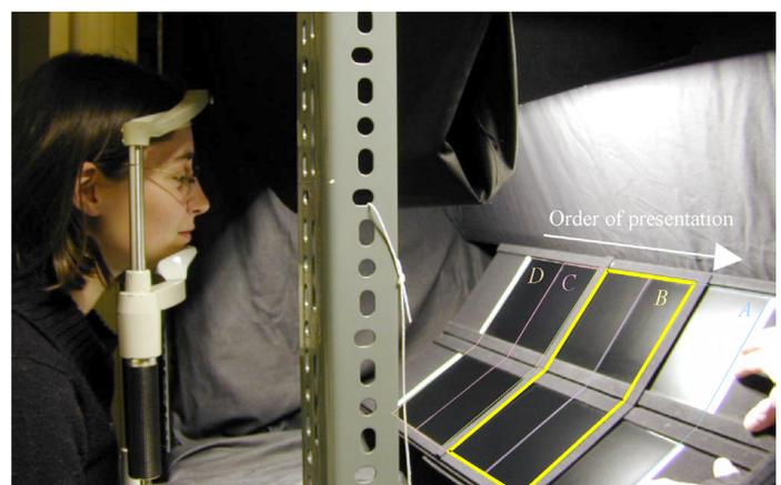
Figure 3. An observer performing the experiment. Observer judges double pair B. Two boards of five samples are presented. The experimenter shifts the boards in front of the observer. The observer judges successively quadruplets A, B, C, and D. Two boards allow the observer to make four paired-comparisons, four by four.
