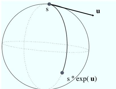
Figure 4: Schematic view of the intrinsic update step used in Newton methods for Lie groups. An unconstrained update  $\mathbf{u}$  is computed on the Lie Algebra and is projected back onto the Lie group through the exponential map.
