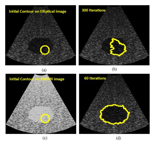
**Fig. 6.** Level set segmentation performed on Elliptical Image (upper row) and the classified image using RMMN (lower row), (a): level set initialization on original image, (b): results after 300 iterations, (c): level set initialization by RMMN classification, (d): results after 60 iterations.
