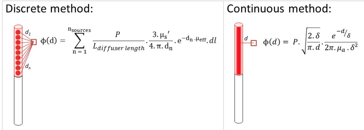
Figure 2: Illustration of the two analytical equations. The discrete method discretizes the diffusing part of the optical fiber as a sum of several light point sources. The continuous method considers the light source as a finite line and computes the fluence rate values using the minimal distance  $d$  from the fiber.
