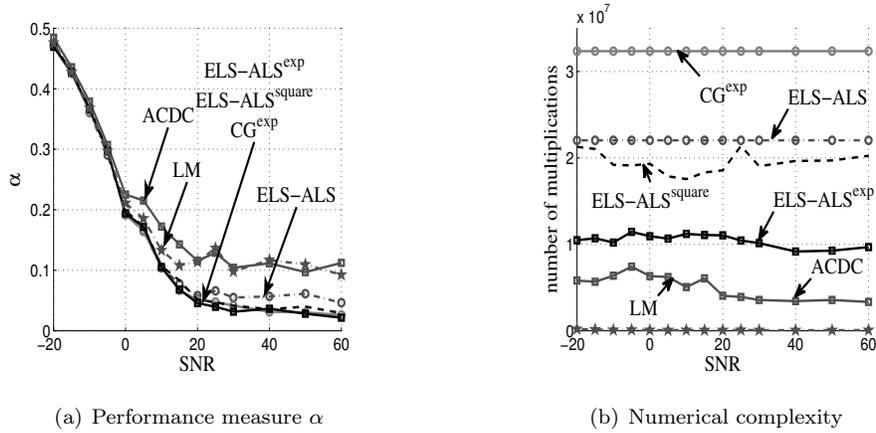
Figure 1: Influence of SNR for a  $(5 \times 5 \times 5)$  array and  $P = 3$  at the output of both proposed methods, called  $\text{CG}^{\text{exp}}$  and  $\text{ELS-ALS}^{\text{exp}}$ , a semi-nonnegative JDC algorithm,  $\text{ELS-ALS}^{\text{square}}$ , a JDC method, ACDC, and two CP methods, namely ELS-ALS and LM.
