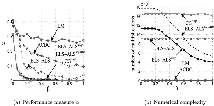
Figure 2: Influence of the collinearity for a  $(10 \times 10 \times 10)$  array and  $P = 4$  at the output of both proposed methods,  $CG^{\text{exp}}$  and  $ELS\text{-ALS}^{\text{exp}}$ , a semi-nonnegative JDC algorithm,  $ELS\text{-ALS}^{\text{square}}$ , a JDC method, ACDC, and two CP methods, ELS-ALS and LM.
