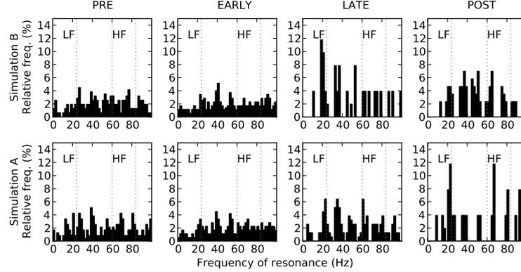
**Fig. 4.** Relative distribution of the frequencies of resonance for each period for Simulations A and B. Bin size corresponds to 2 Hz intervals. The dotted lines delineate the limits of *LF* and *HF* bands.
