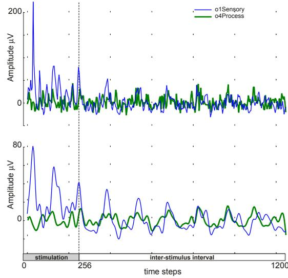
**Fig. 2.** Evoked potentials averaged over 50 trials obtained from  $u1Sensory$  (blue solid trace) and from  $u4Process$  (green dotted trace) *Ubidules* during the *EARLY-learning* stage. The stimulus was applied during 256 time steps. The upper panel displays the raw evoked potentials and the lower panel shows the signals smoothed by a Blackmann smoothing window in order to emphasize the low frequency components.
