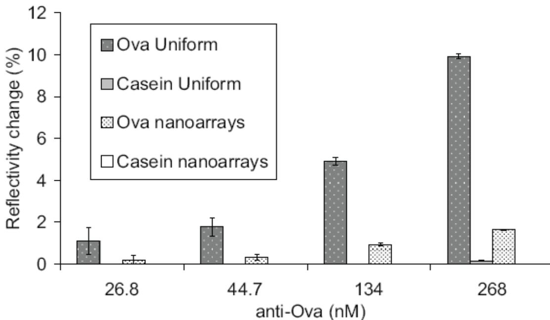
**Fig. (4).** SPRi signals related with the bio-interactions on SiOx nanoarrayed and uniform PPy surfaces. Different concentrations of anti-Ova were successively injected on a SPR chip grafted with Ova (assay), Casein (control).
