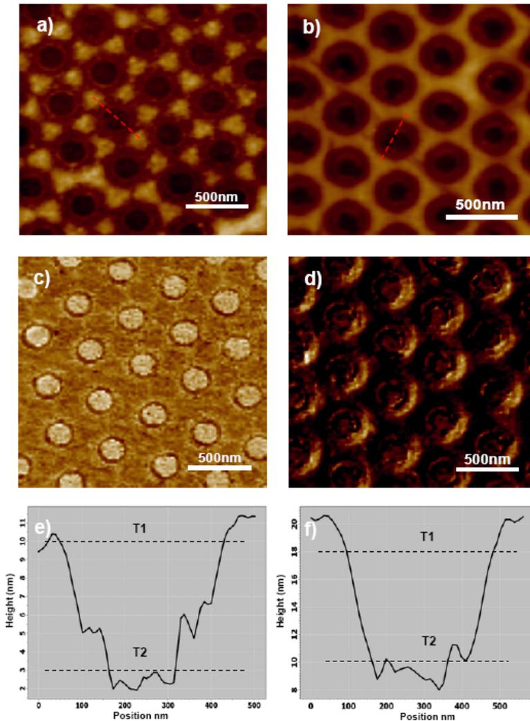
**Fig. (2).** AFM analysis of the nanotemplates: **a-c-e)** 10 nm SiO<sub>x</sub> and **b-d-f)** 10 nm SiO<sub>x</sub> + 10 nm of PEO; **a-b)** topographic images, **c-d)** corresponding phase images and **e-f)** height profiles along the dot lines. [a) vertical scale 0-20nm; c) color scale: -80 to 100; b) vertical scale 0-25 nm; d) color scale: -10 to 00].
