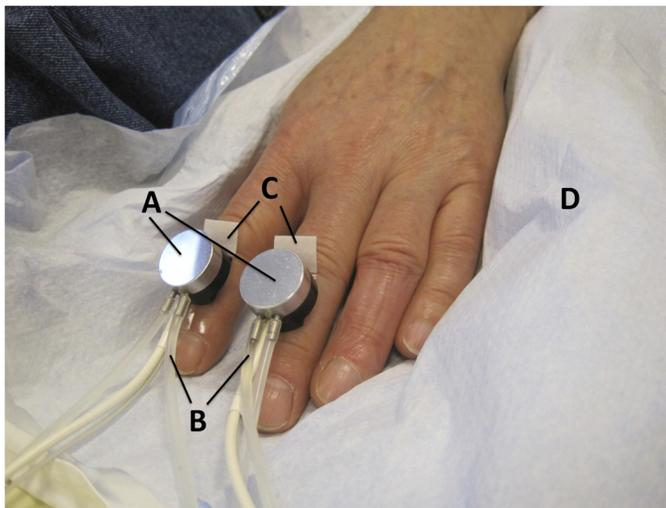
Fig. 1. Single-point laser Doppler probes (A) with a liquid cooling system made of silicon tubes (B). C: probes were fixed with double-sided tape. D: a vacuum cushion was used to decrease artifacts associated with arm movements.
