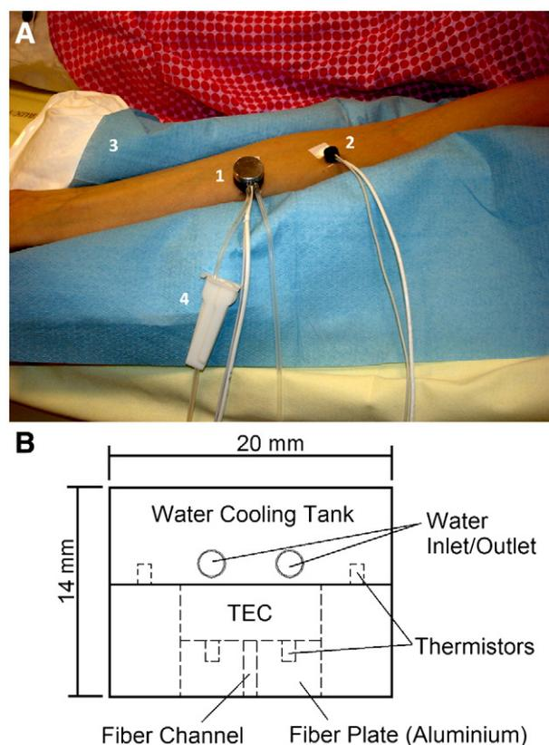
**Fig. 1.** (A) LDF cooling probe prototype (1) and 5-cm control site probe (2). A vacuum cushion (3) was used to decrease artifacts associated with arm movement. The liquid cooling system is made of silicon tubes with a cutting wheel (4) to regulate water flow. (B) Schema of the cooling probe prototype. TEC: thermoelectric cooler.
